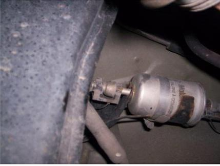
6. Clip your 5/16 tool of the lines on the fuel filter. Once it is on hard fuel filter line, pull it into the main fuel line until you hear a click.
