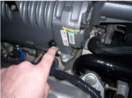
3. Remove the black cap and depress pin with a phillips screw drive. You may want to cover with a rag. Depending on how long the car has been sitting will effect the amount of pressure in the fuel rail.
