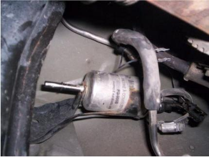
10. Once the clamp is off, pull the filter up to remove from bracket.
