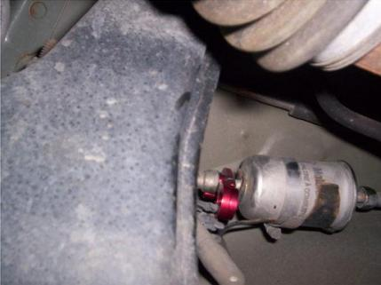
7. Pull the tool into the main fuel line. You may need to push the filter with your knuckle for leverage. May need to work the tool up and down. Be patient, the line will come off. **Note that the fuel line ends are spring loaded. The tool pushes the spring over the flare.**
