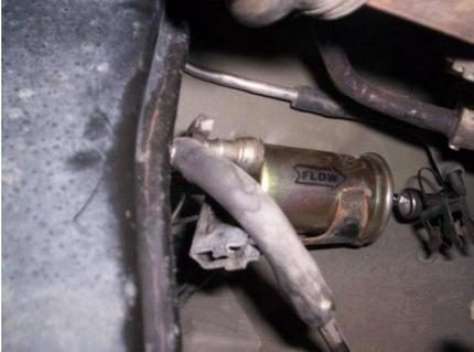
12. Slide the metal clamp on the filter and bracket and tighten down.
